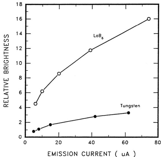
**Figure 4.** Relative brightness recorded from screen current versus total emission current for 5 Brightness settings with the emission at saturation. Data from Philips EM-420 TEM with LaB<sub>6</sub> and tungsten cathodes.
