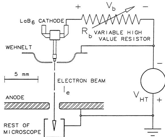
Figure 3. Basic electrode geometry of triode electron gun, showing auto-bias resistor R<sub>b</sub> and operating bias V<sub>b</sub> = R<sub>b</sub> × I<sub>e</sub> where I<sub>e</sub> is the total emission current.
