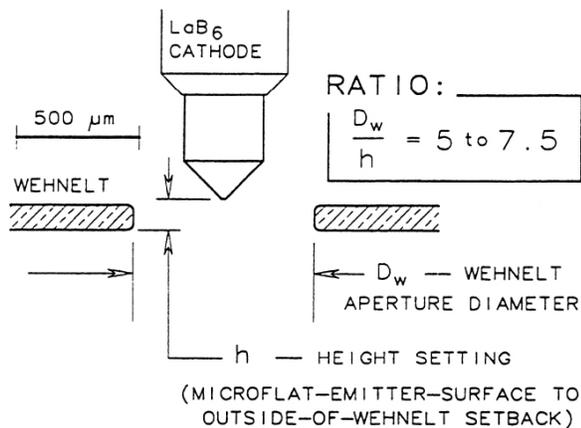
**Figure 1.** Scale drawing of KPI ES-423E LaB<sub>6</sub> Cathode set at height 125 μm in a Wehnelt of 100 μm thickness with an aperture diameter of 750 μm. The ratio of D<sub>w</sub> to h is 6, typical of that required for high brightness performance.
