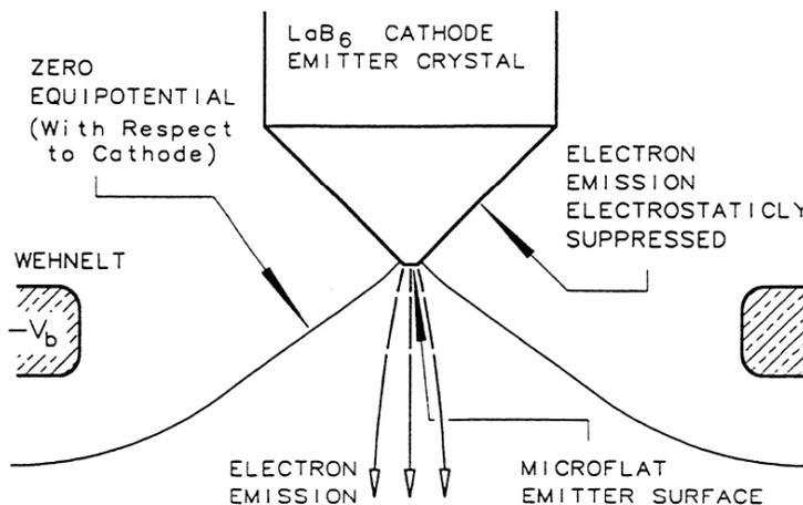
**Figure 2** Intercept of the zero-equipotential (measured with respect to the cathode) on the tip of a truncated LaB<sub>6</sub> cathode, defining the area of emission at saturation (optimum) bias.
